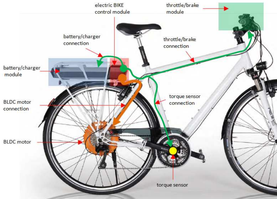
Figure 1. Electric BIKE components.
