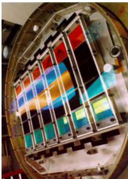
Figura 8.18. Telescopul Sloan Digital Sky Survey, cu senzori CCD, sursa https://en.wikipedia.org/wiki/Charge-coupled_device
