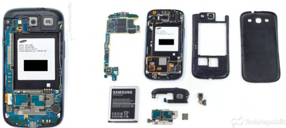
Figura 10.7. Telefon Samsung Galaxy S3 dezasamblat, sursa http://www.slideshare.net/YongHeuiCho/4smartphone-hw-architecture
