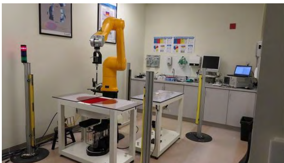
Figura 13.6. Sistem de măsurare SAR, sursa https://www.ic.gc.ca/eic/site/ceb-bhst.nsf/eng/h_tt00084.html
