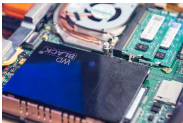
Figura 3.9. Hard disc hibrid WD Dual Black, sursa
