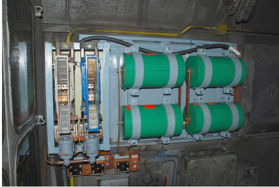
Fig. 4. The power system (supercapacitors, mechanical and solid state relays) mounted in the engine compartment
