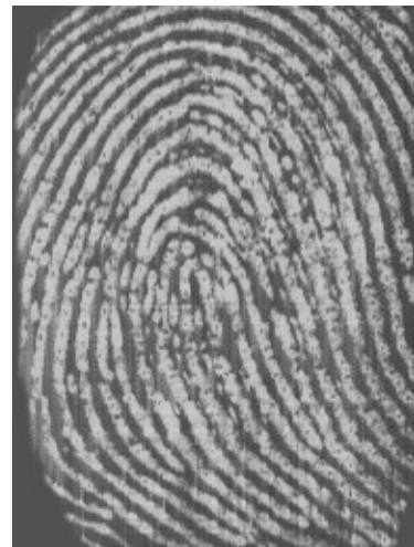
Figure 2. Fingerprint image captured with a capacitive sensor
