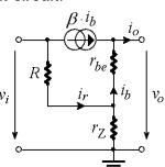
The output resistance is much smaller than for the zener regulator, the dynamic resistance of the zener beeing reduced by the high  $\beta$  factor (and  $1/g_m = r_e$  has a very low value).
