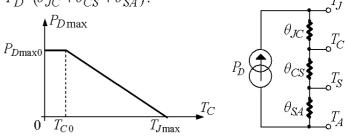
The  $P_{D\,\mathrm{max}}$  level of power dissipation cannot be achieved in practice; it would require an infinite sink and  $T_A \leq 25^{\circ}\mathrm{C}$ ). Normally  $P_{D\,\mathrm{max}}$  watts transistors can dissipate about  $0.4P_{D\,\mathrm{max}}$  for a reasonable heatsink.
