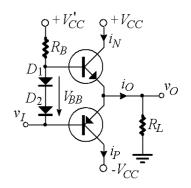
contact with the output transistors, theirs temperature will increase by the same amount as that of  $Q_N$  and  $Q_P$ . Thus  $V_{BB}$  will decrease at the same rate as  $v_{BEN} + v_{EBP}$  with the result
