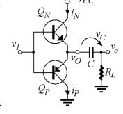
For the positive half cycle of the signal,  $v_i > 0$ ,  $Q_N$  is ON and the current path (for  $i_N$ ) is from  $V_{CC}$  through  $Q_N$ , C,  $R_L$  to ground. The capacitor C is slightly charged (because the conduction time, T/2, is much less than the circuit time constant,  $R_LC$ ).
