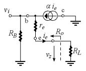
**S7 – P2**. *a)* Determine the voltage gain and the input and output resistances for the amplifier in figure; consider:  $I_C = 2 \text{ mA}$ ,  $\beta = 200$ ,  $V_T = 25 \text{ mV}$ ,  $(V_{BE} = 0.7 \text{ V})$ .
