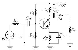
The signal source is coupled to the base of the transistor through coupling capacitor  $C_B$  and the output signal at the collector is coupled to the load,  $R_L$ , through another coupling capacitor  $C_C$ .
