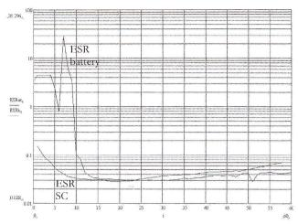
Fig. 7 Short time variation of ESR during the first 600 ms after begin of the starting process with logarithmic scale on Y axis - (blue represents ESR variation in time for batteries and red represent the ESR variation in time for supercapacitors – the measurement was obtained using a shunt with  $60 \mathrm{m}\Omega$  resistance)
