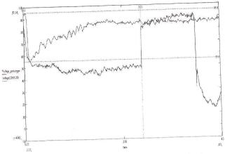
Fig. 5 Voltage variation during the starting process for the LDH1250HP (blue), and the voltage variation (red) during the starting process for the prototype LDH1250 endowed with the new energy management system
