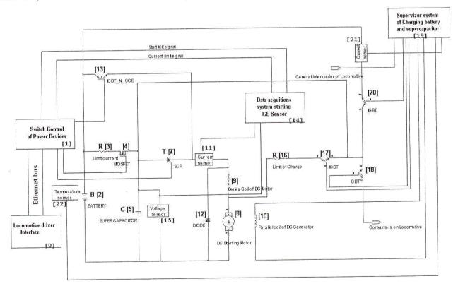
Fig. 3 Scheme of energy management system mounted on locomotive LDH1250HP
