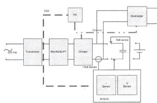
Fig. 1 Scheme of the test bench
