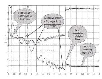
Fig. 8 Current and Voltage variation during the starting process (X axis: time is measured in seconds)
