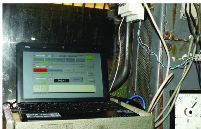
*An electric starting system installed on locomotive. The system include two components: the locomotive driver console (left) and the embedded systems dedicated for the main subsystems. The picture on the right shows the box of supercapacitors and the afferent control systems linked to console by an Ethernet bus.*
